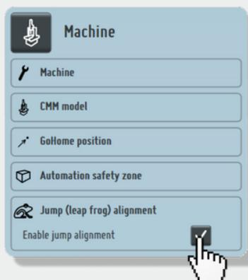
Once enabled, you can define jump alignment from the Measuring port.
