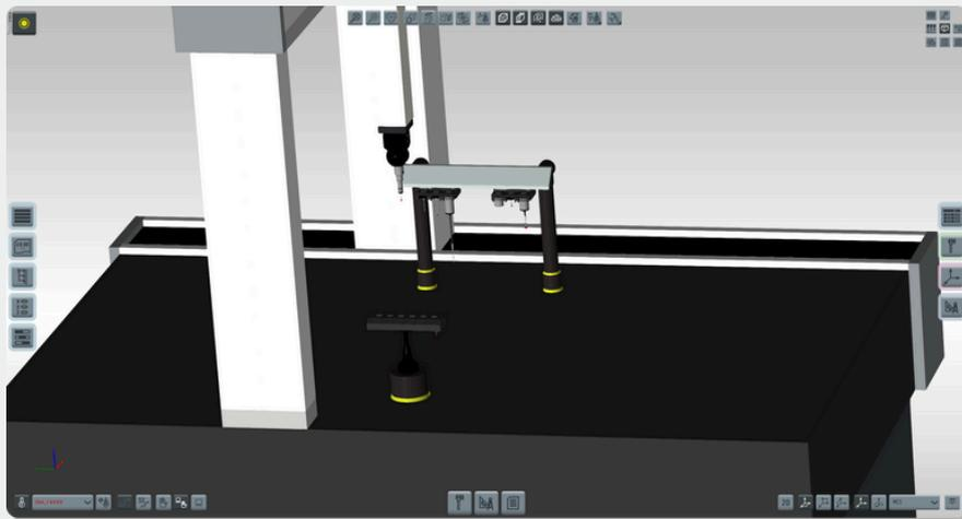
And we have improved the graphical model of all changer racks and more realistic design of calibration spheres.
