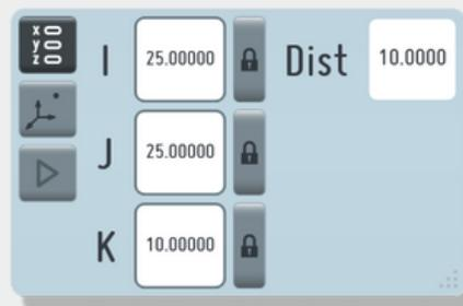
Like simple GoTo, you can input incremental GoTo's and press play to execute the operation.
