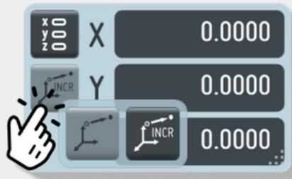
You can select Incremental GoTo by right-click or tapping and press hold the GoTo button on the Actual coordinate window.
