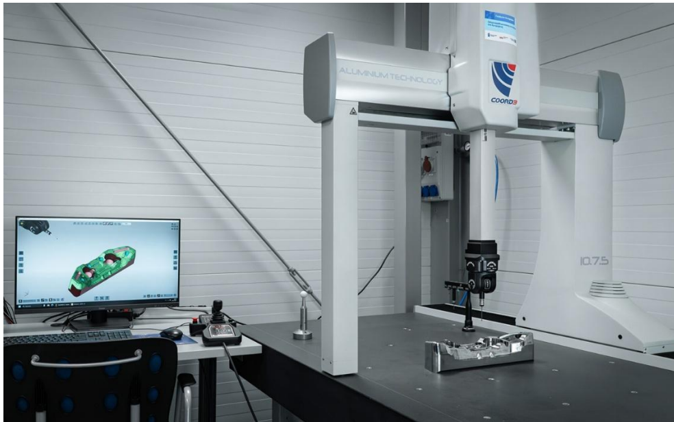
Figure 3 - Stjorsen metrology room: Coord3 Ares 10.7.5 equipped with PH20, TP20 and TouchDMIS
