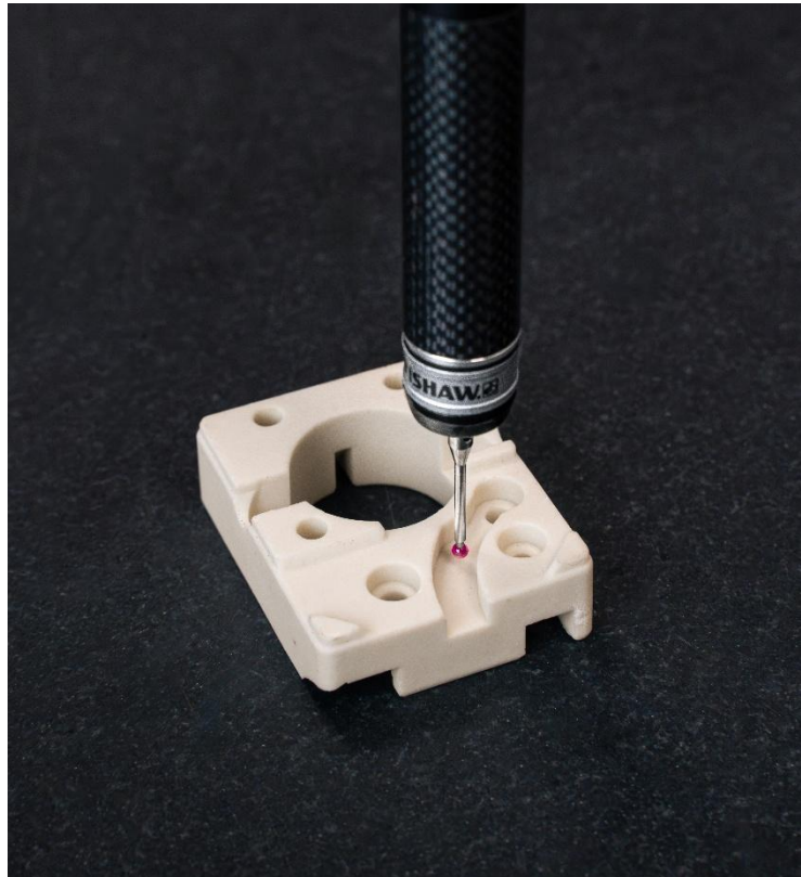
Figure 2 - Inspection of ceramic part in Stjorsen
